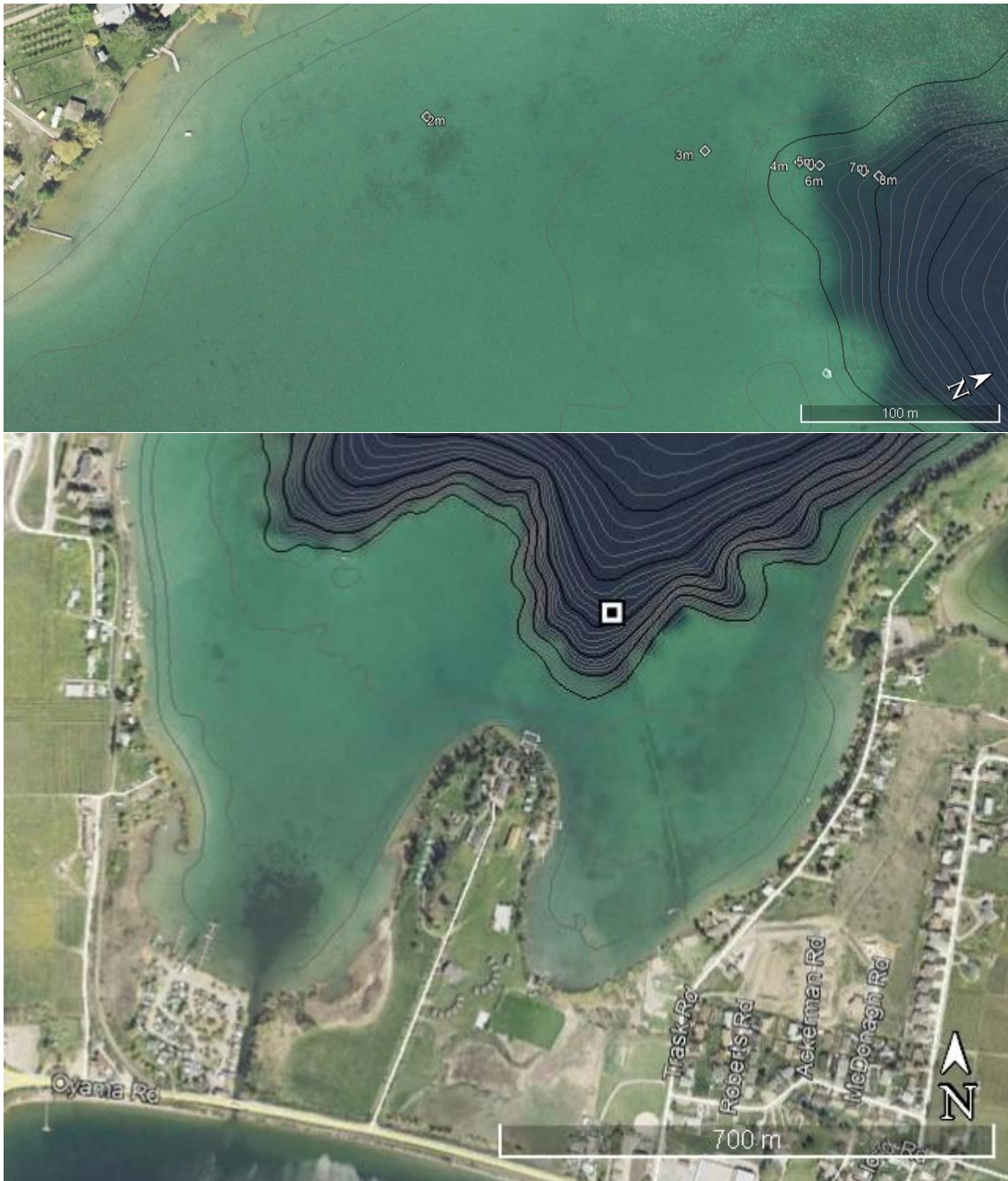
Figure 1: Map of buoy locations and bathymetry contour lines in the south bay of Kalamalka Lake (top) and location of DLC intake (bottom)
